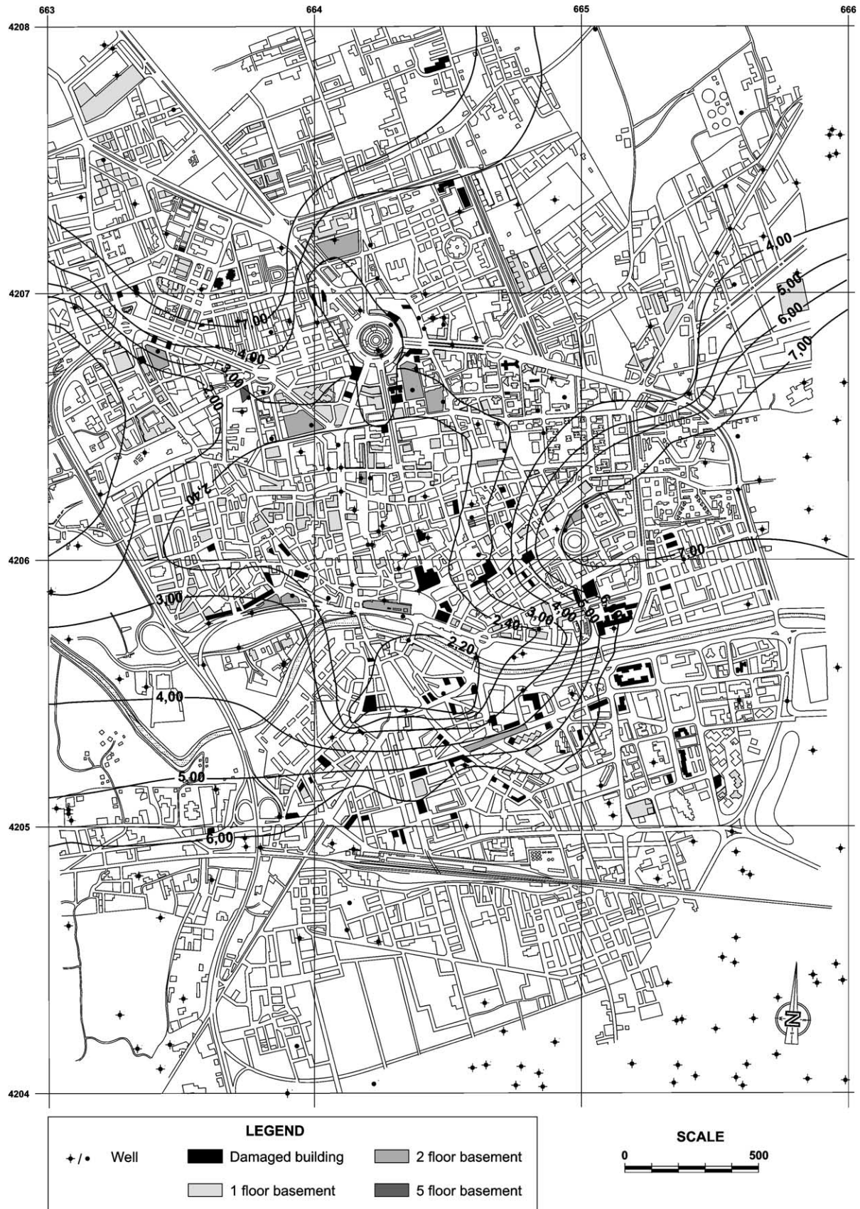
Fig. 4. Inventory map of damaged buildings, wells and basements showing subsidence values in the city of Murcia estimated using numerical models for the 1993–1998 period (based on Mulas et al., 2003 and Vázquez & De Justo, 2002). Settlement values are in cm.
