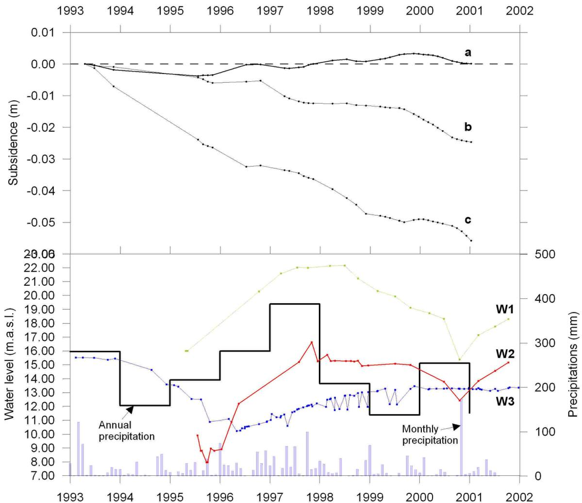
Figure 2. Deformation evolution at three different points of the studied area, correlation with three different piezometers (see location in Figure 1), and monthly precipitations.
